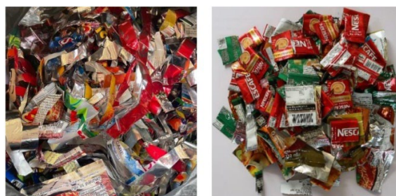
Figure 1 ML packaging as feedstock with raw material size of 4 × 4 cm.
