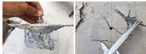
Figure 10 Failure pattern in Pull-Out test
