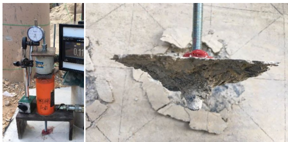
Figure 9 Picture of the disaster in pulling anchors from the test yard in the Concrete Break Out format.
