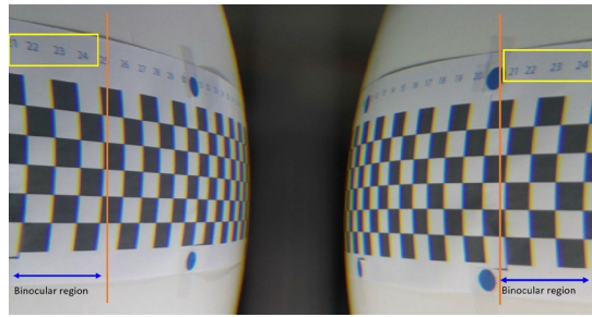
Figure 7 Wide target used to illustrate scene setup and prism distortion.
