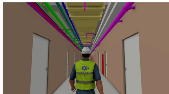
Revit + Fuzor collision detection optimized corridor.
