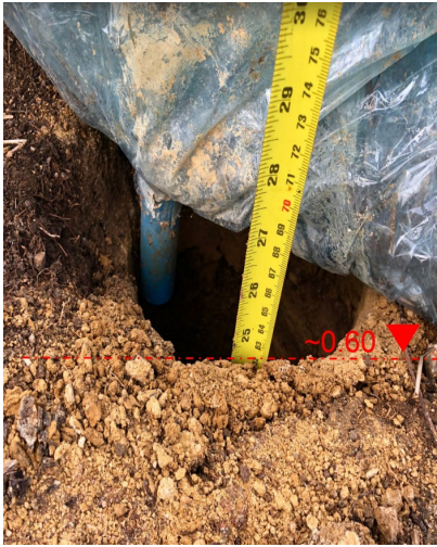
Figure 10. Depth measurement of a hole filled by KOH flakes and water after 2 weeks.
