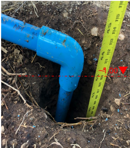
Figure 7. The depth of Hole 1 (KCl solution) was only 1 m after 2 weeks.
