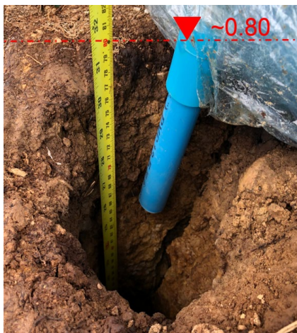
Figure 11. The remaining depth of water-soaked hole followed by KOH flakes 20% by volume was about 80 cm.
