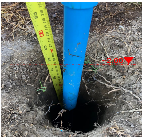
Figure 8. The depth of Hole 2 (KOH) still remained at about 2 meters.
