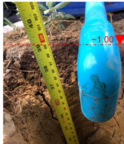
Figure 9. Depth of \text{KNO}_3 hole was measured about 1 m after 4 weeks.
