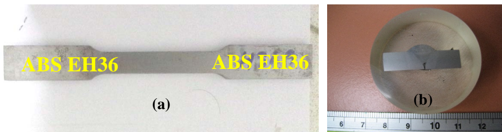
Figure 2 Specimen of ABS EH36 (a) for tensile test method (b) for hardness test method, OM, SEM and EDS
