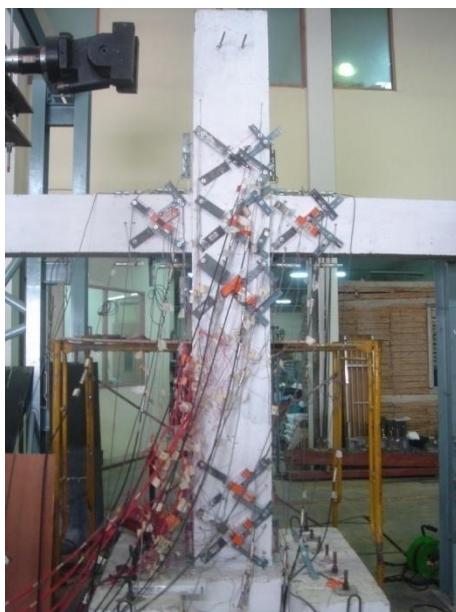
Figure 5 Instrumentation of specimen
