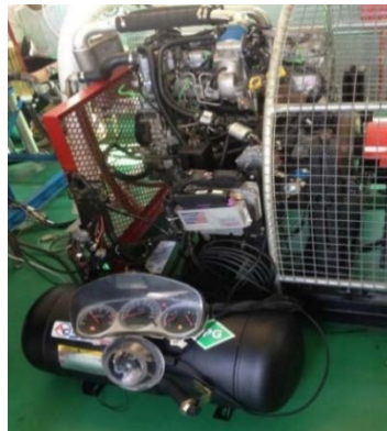
Figure 1 The LPG injection system installed with the engine
