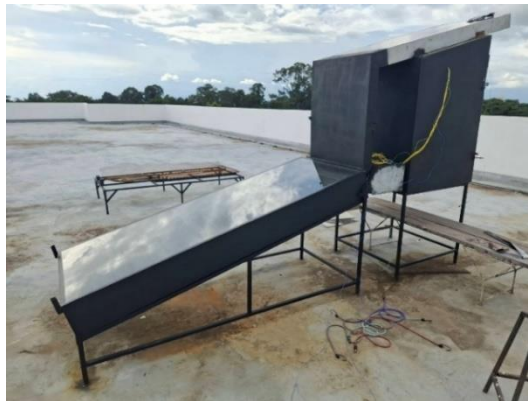
Figure 2 Photograph of the experimental photovoltaic-thermal solar dryer system.
