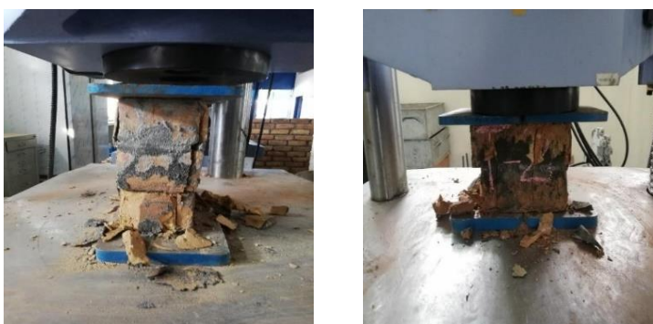
Figure 5 Vertical splitting failure of brick prisms
