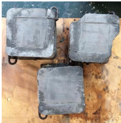
Figure 3 Concrete cubic mold sized 10x10x10 centimeters
