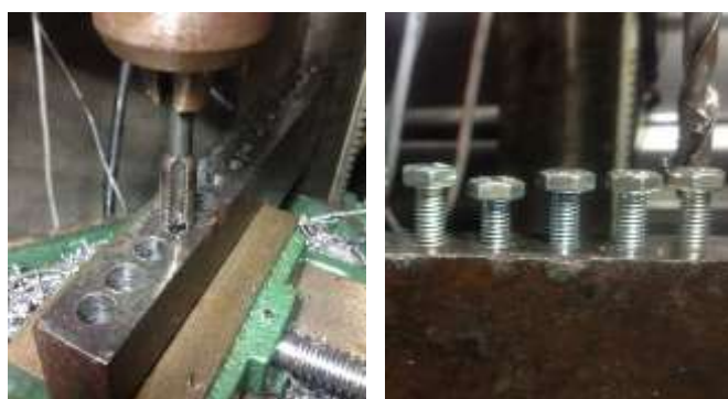
Figure 8 Thread depth inspections
