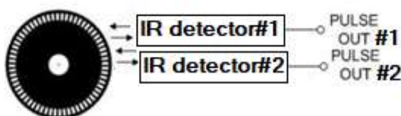
Figure 1 Working principle of rotation encoder.
