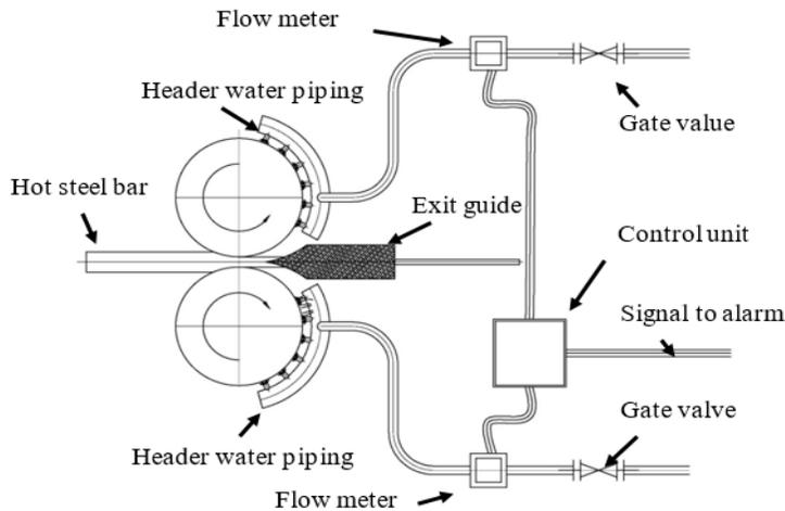
**Figure 12 Roll cooling system with sensor devices**
