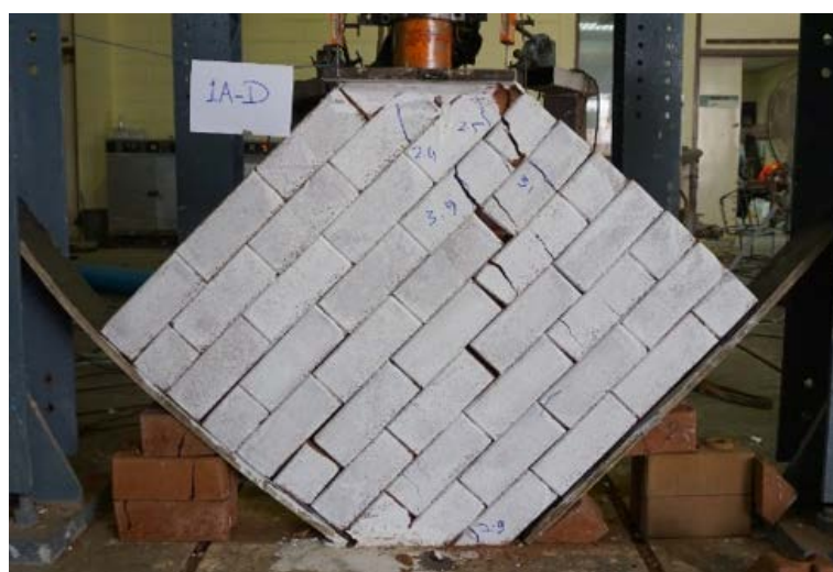
Figure 16 Failure mode of wall specimen 1-D
