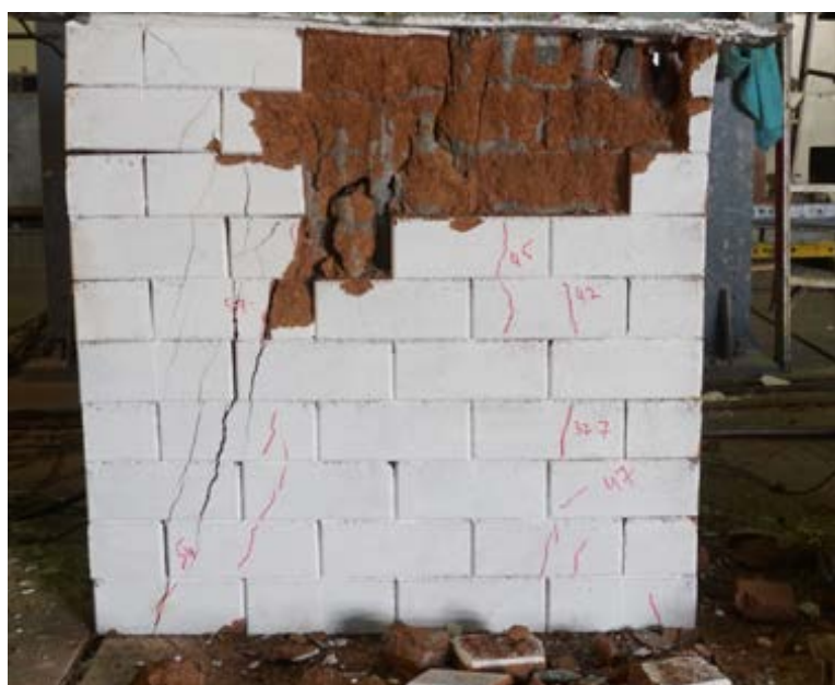
Figure 15 Typical failure mode of cement grouted reinforced walls (Axial compression)
