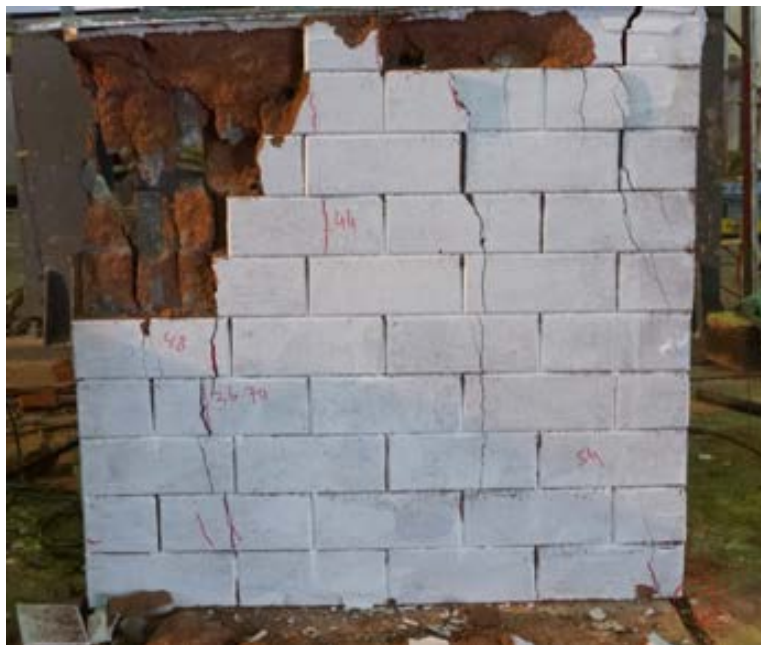
Figure 14 Typical failure mode of cement grouted un-reinforced walls (Axial compression)
