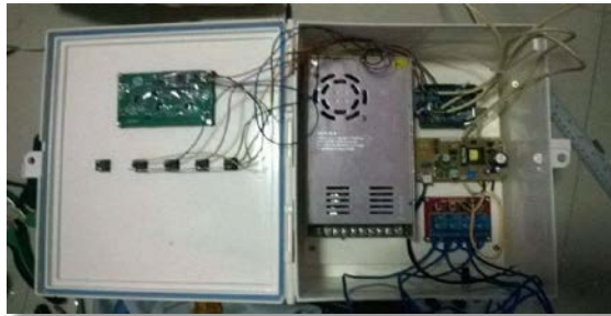
Figure 8 Roller drive trainer with adjustable three-levels by microcontroller with material in the box
