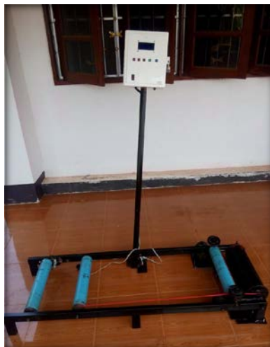
Figure 9 Roller drive trainer with adjustable three-levels by microcontroller structure
