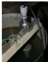
Figure 5 Soil Moisture Sensor, EC (pH) Sensor and Solenoid water valve installation
