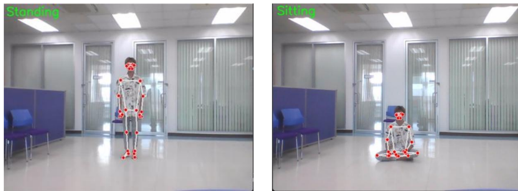
Figure 4 Example of 33 body landmarks detected in both standing and sitting postures
