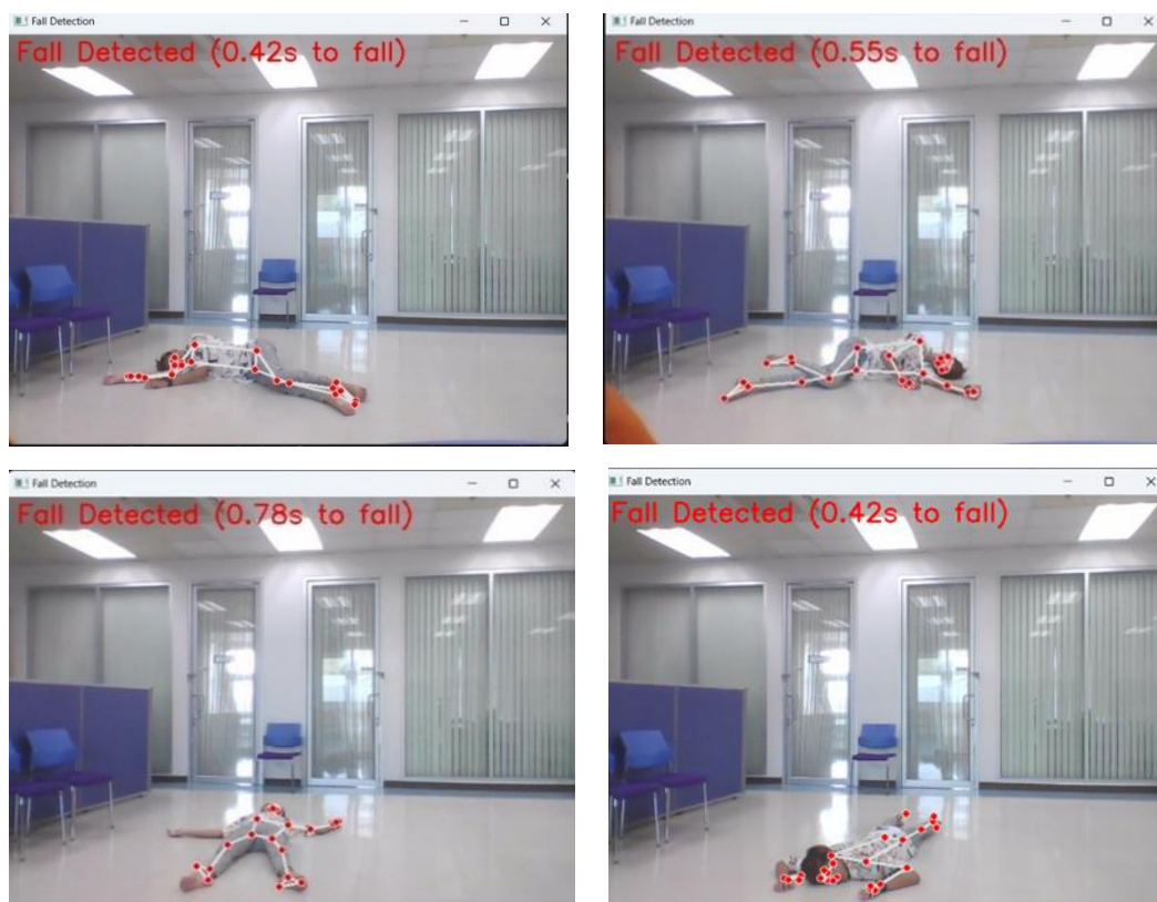
Figure 5 Simulation results of four fall types (left, right, forward, and backward) with recorded fall duration
