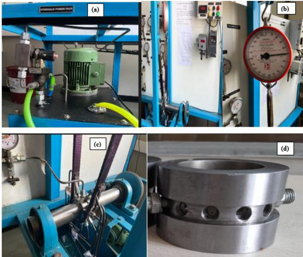
Fig. 3. (a) The power pack unit; (b) The arrangement for the experiment; (c) The setup for pressure sensors, along with load and bearing installation; (d) The test bearing equipped with twelve evenly spaced openings for mounting pressure sensors.
