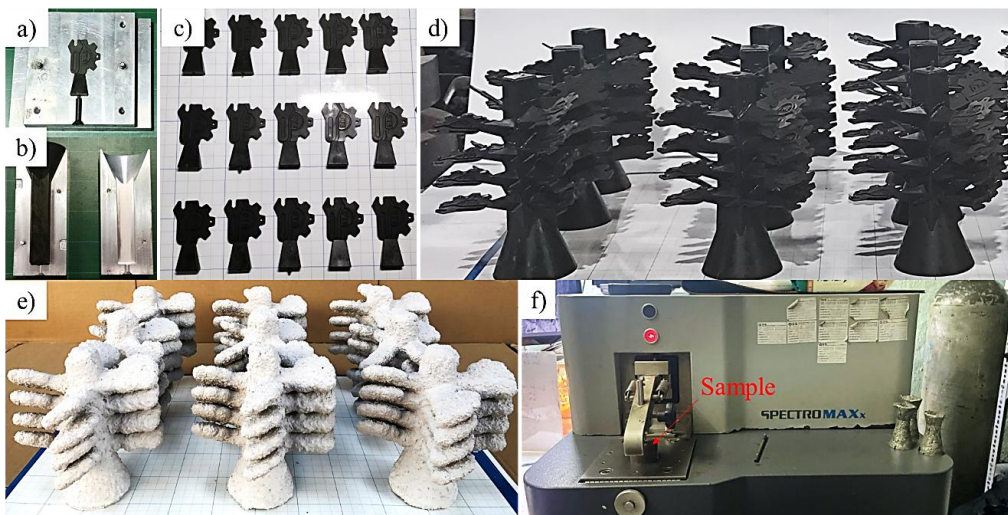
Fig. 5. Experiment process (a) mold for pattern, (b) mold for pouring cup and pouring basin pattern, (c) pattern, (d) tree of pattern, (e) mold shell, and (f) SPECTROMAXx spark optical emission spectrometry machine.
