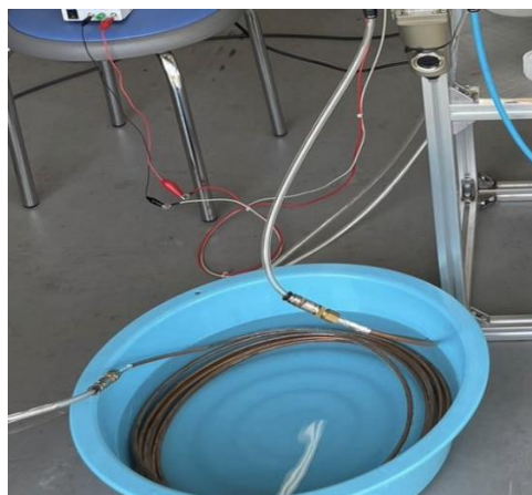
Fig. 9. Appearance of the cooling section.
