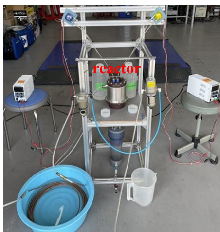
Fig. 3. Actual appearance of the H_2 generation system.
