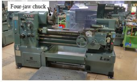
(a) General-purpose lathe used in the experiment (b) Clamping the workpiece
