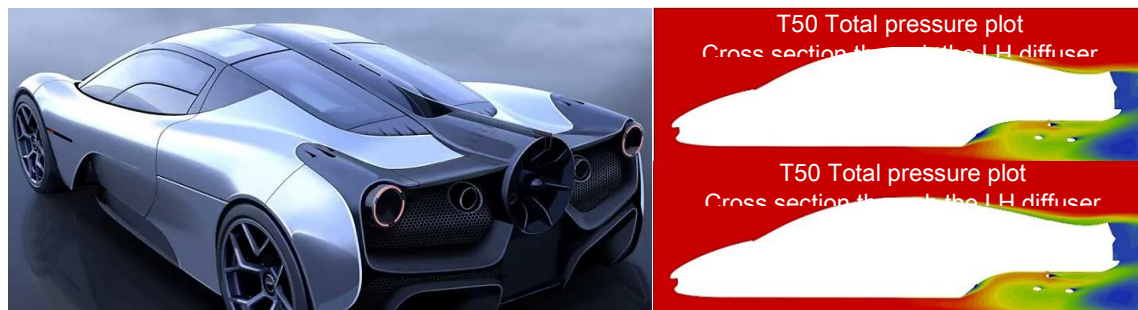
Fig. 2. Reduction of wake and flow reattachment over the rear of GMA T50 due to the induced flow by the rear fan [2]
