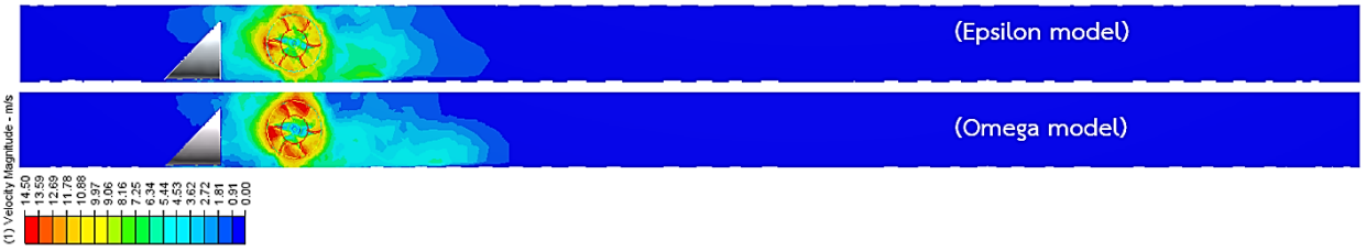
Fig. 16. Comparison of rotational velocity fields at flow rates of 0.00150 m 3 /s.
