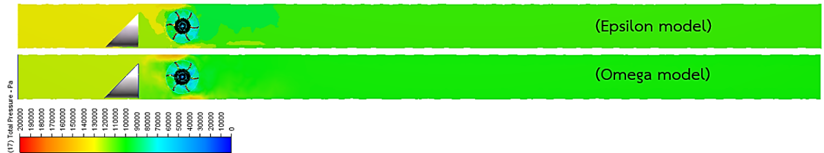
Fig. 20. Comparison of pressure fields at flow rates of 0.00134 m 3 /s
