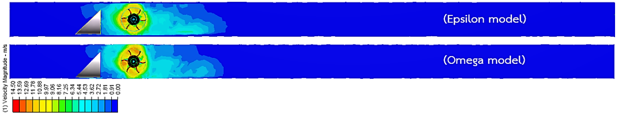
Fig. 15. Comparison of rotational velocity fields at flow rates of 0.00134 m 3 /s.
