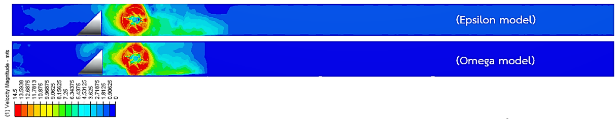
Fig. 18. Comparison of rotational velocity fields at flow rates of 0.00184 m 3 /s.
