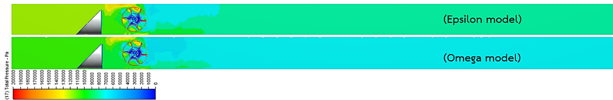
Fig. 24. Comparison of pressure fields at flow rates of 0.002 \text{ m}^3/\text{s}
