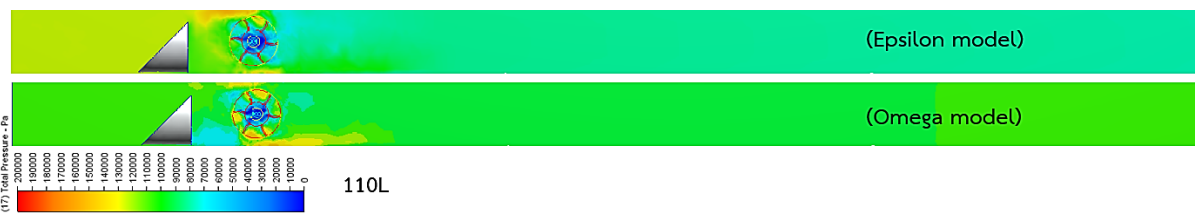
Fig. 23. Comparison of pressure fields at flow rates of 0.00184 m 3 /s
