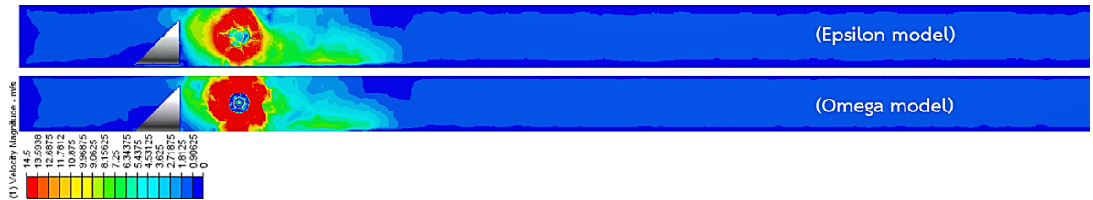
Fig. 19. Comparison of rotational velocity fields at flow rates of 0.00200 m 3 /s.
