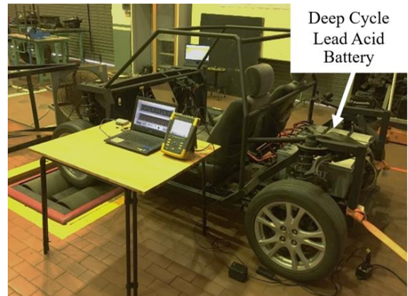
(b) a car powered by deep cycle lead-acid battery
