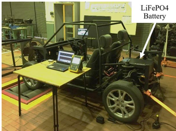
(a) a car powered by lithium-iron phosphate battery
