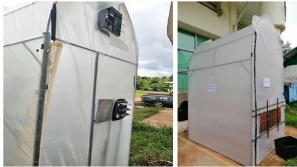
Fig. 2. The evaporative cooling system and fans.
