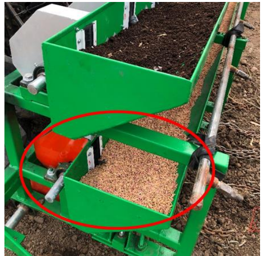
Fig. 7. Prototype of seed swivel disc vertical connect to sowing machine
