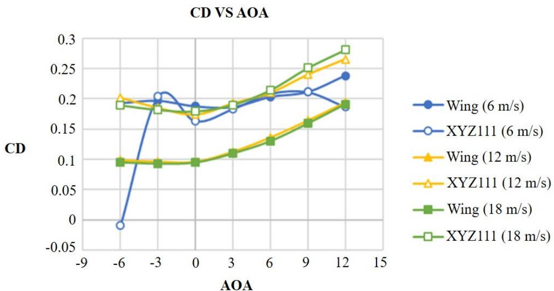
Fig. 6. The drag coefficient of clean wing and wing with propellers XYZ111 configuration vs AOA
