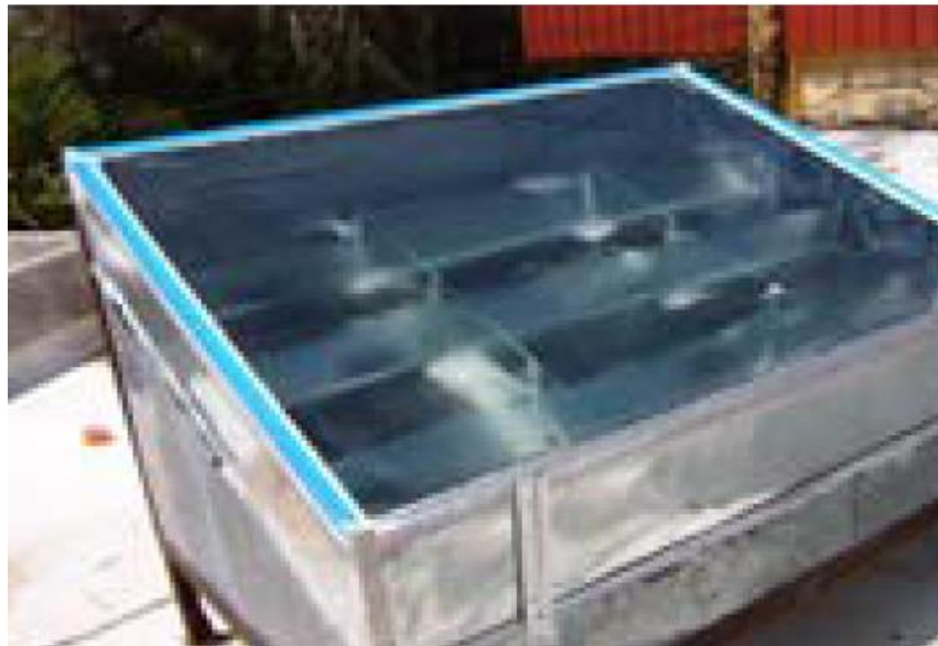
Fig. 1. a) Experimental setup for the double slanted-glass distillation unit: 1. Stand for the distillation unit, 2. Compressed wood partition, 3. Insulator, 4. Glass screen, 5. Glass partition for upper gutter, 6. Heat absorber, 7. Inlet water, 8. water inside the upper and bottom layer and 9. Outlet for distilled water. b) Photograph captured of the solar-based distillation unit employed in the experiment.
