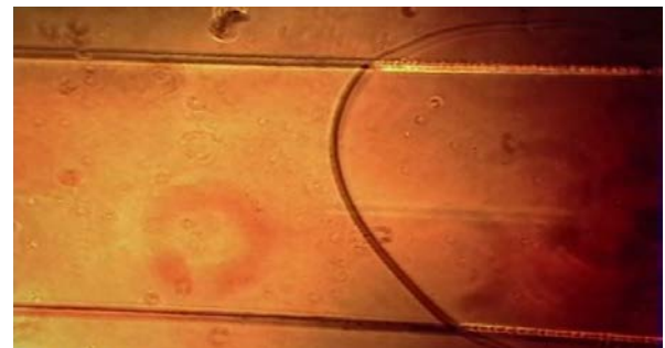
Fig. 4 Slip flow profile occurred at entrance of a leak LOC because of high friction force at boundaries.
