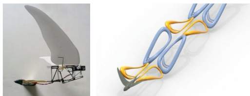
Fig. 4 MAV model inspired particularly by swift, hoping to improve energy efficiency beyond normal fixed wing MAVs. Also shown is the impression of the wake in slow forward flight [10]
