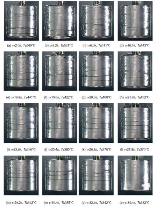
Fig. 3 Photographs of vapor film covering a vertical finite-length cylinder
