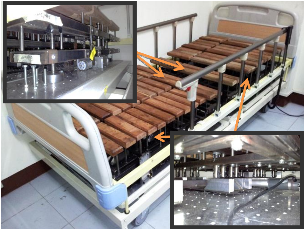
Fig. 9 Installation of the anti-bedsore bed with a general hospital bed and the mechanisms within the anti-bedsore bed.
