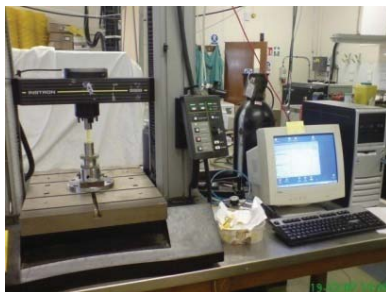
Fig.9 The uniaxial compression test using the INSTRON machine 5543.
