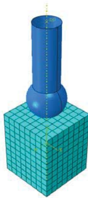
Fig. 4 The assembly between silicone model and indenter.
