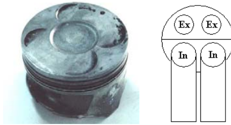
Figure 1. Test piston with flat type and configuration of intake port with parallel type
