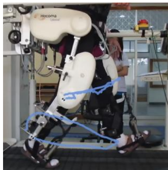
Fig. 1. Path of Ankle Movement in Lokomat (Experiment).
