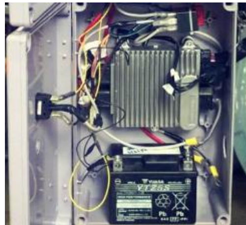
Fig. 7. The Engine Control Module used for controlling the working status of the ACG.
