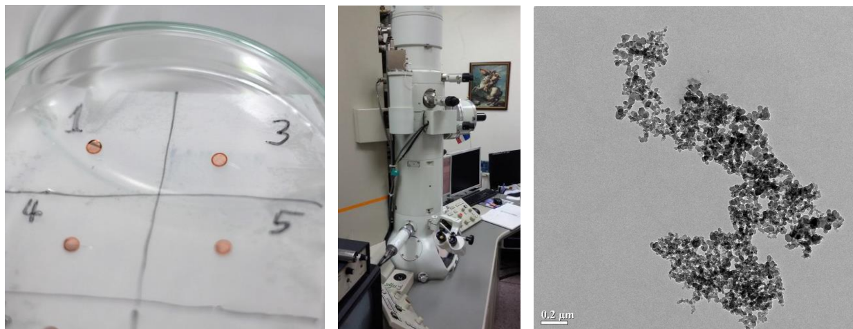
Fig. 2. Carbon black and soot powder prepared in copper grid for Transmission Electron Microscopy.
