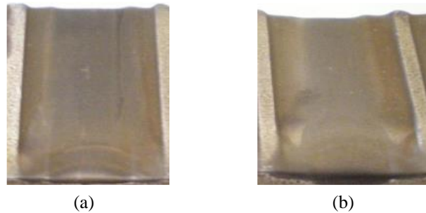
Fig. 7. Actual slots machined by the hollow tool with outer diameter (a) 12 mm and (b) 14 mm.
