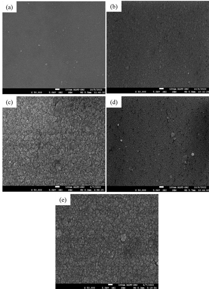
**Fig. 5** FESEM images of AlGaIn at different sputtering pressures (a) 1 mTorr, (b) 3 mTorr, (c) 5 mTorr, (d) 7 mTorr, and (e) 10 mTorr.
