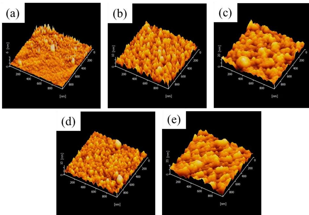
**Fig. 4** AFM images of AlGaIn films at different sputtering pressure (a) 1 mTorr, (b) 3 mTorr, (c) 5 mTorr, (d) 7 mTorr, and (e) 10 mTorr.
