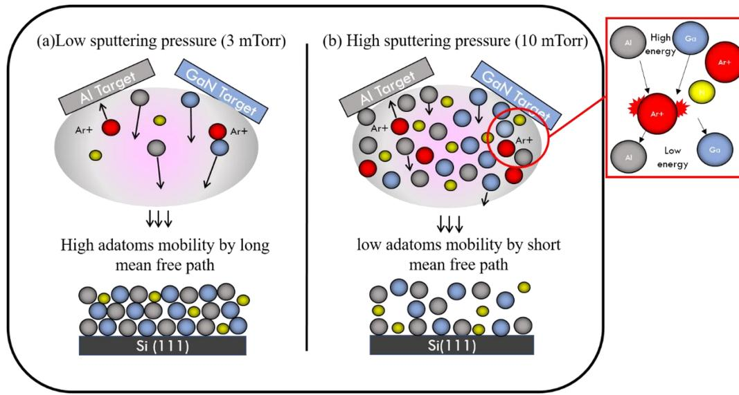
**Fig. 6** Mechanism of sputtering pressure (a) low sputtering pressure, and (b) high sputtering pressure.
