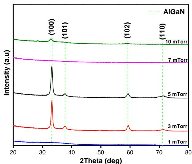
**Fig. 2** XRD pattern of AlGa<sub>N</sub> thin films at different working pressure
