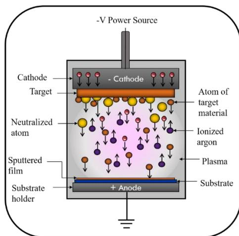
**Fig. 1** Mechanism of the co-sputtering technique
