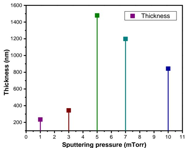
**Fig. 3** Thickness of AlGaIn thin films at different sputtering pressure.
