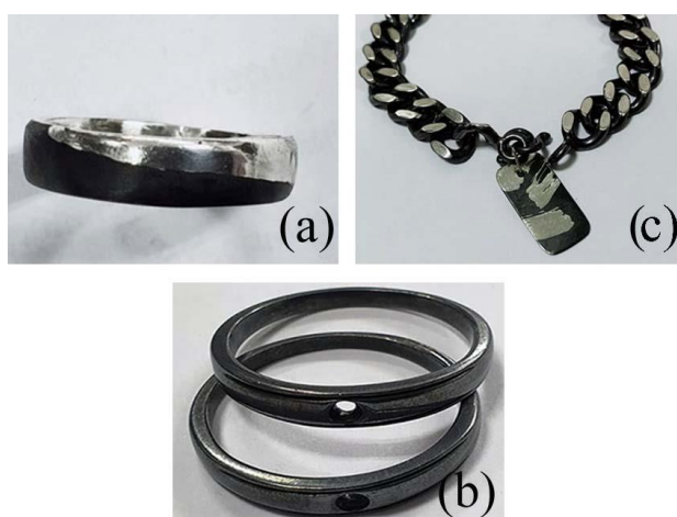
Fig. 9 Silver jewelry products coating with \text{Ag}_2\text{S} films, (a), (b) ring and (c) chain.
