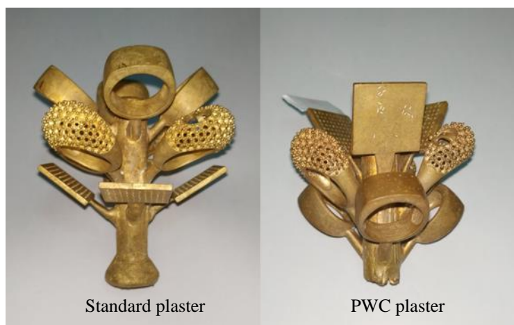
Fig. 6 Jewelry product casting by Standard plaster (left) and PWC plaster (right).
