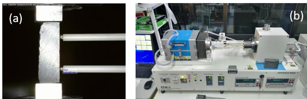
Fig. 1 Measurement system of thermoelectric properties (ZEM-3, ADVANCE RIKO, Inc.).
