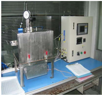
Fig. 23 Instron Set (Model TC-48-20) to Test thermal conduction and thermal resistance
