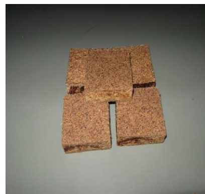
Fig. 10 Cutting Parts to be Tested for Physical Properties, size 50 × 50 mm.
