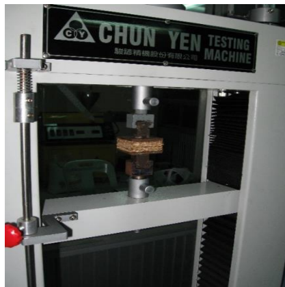
Fig. 19 Instron Set (Tensile Iestel Model 5560), to Test Tensile Strength being Perpendicular to the Surface and Bond Strength of Screws
