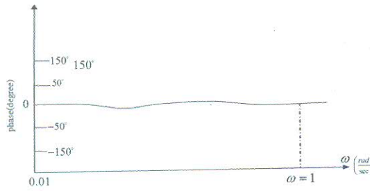
Fig. 6. Phase characteristics of the gain slope equalizer.
