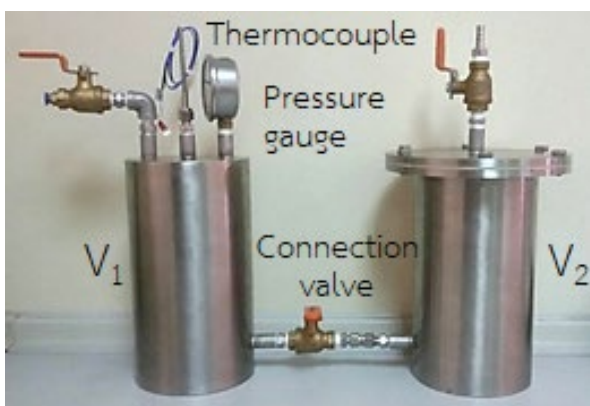
Fig. 2 In-house-made gas expansion pycnometer
