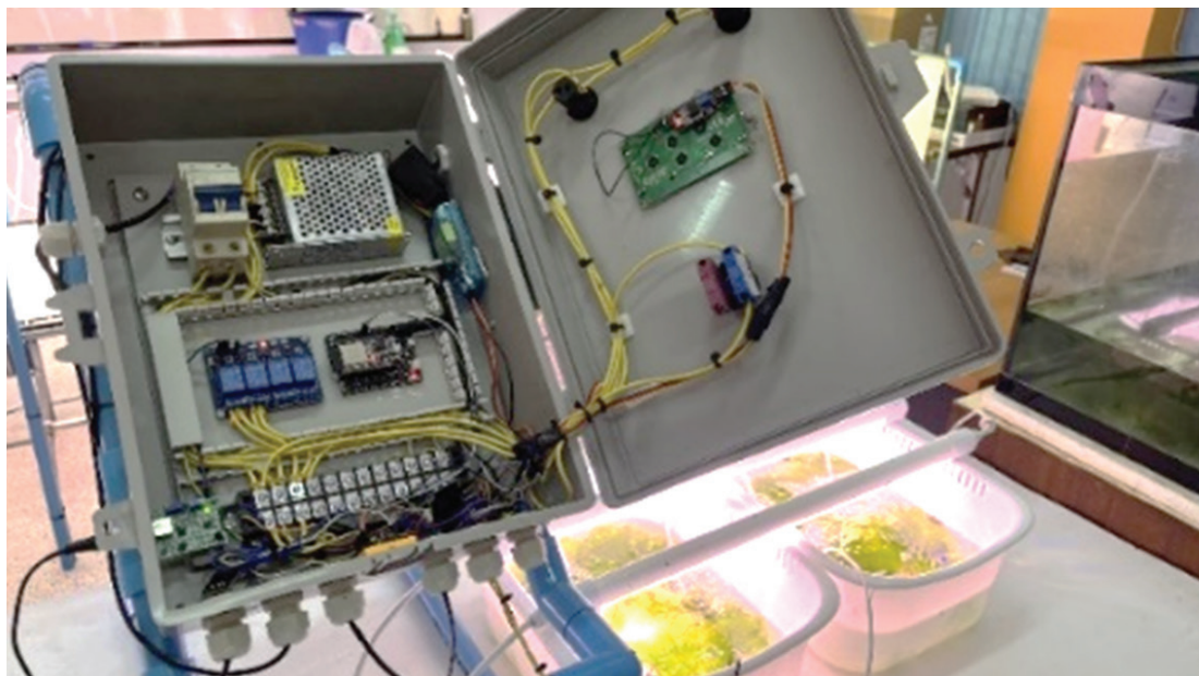
Figure 3. Prototype of IoT-based sea lettuce cultivation system
