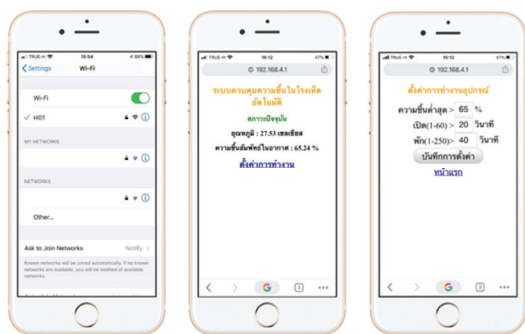
Figure 5. Connecting to Wi-Fi from the set 1 of devices using a smartphone and the user interface displayed on the web browser
