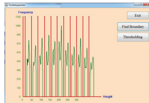
Figure 25 Searching the optimal points along the height of the image.
