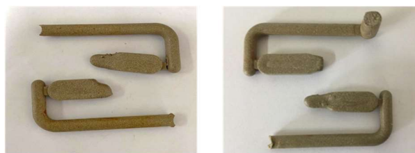
Figure 3 Incomplete shape of green parts with mixture ratio of formula No. 1 and 2.
